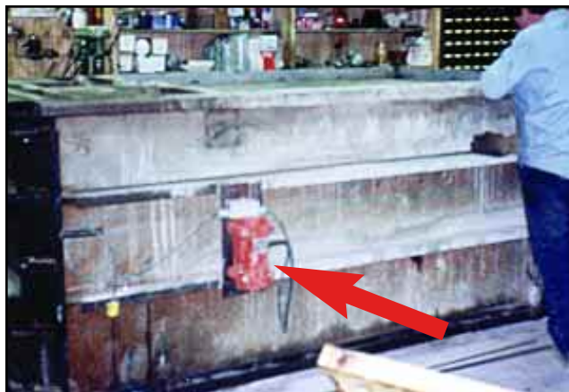
Model US-1600 permanently mounted on 5500 lb. mold.
