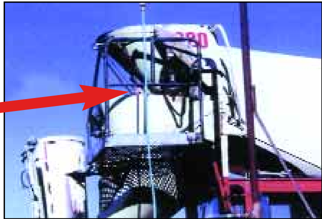
VIBCO VS-250 air vibrator mounted on the charge hopper of a front discharge mixer truck. (Complete kit available.)
