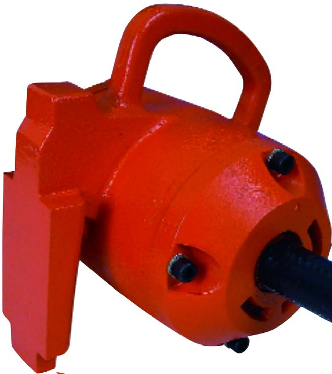
Use a hammer on top strike pad to secure or bottom strike pad to remove wedge in female bracket.
